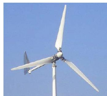
Figure 2: Horizontal axis wind turbine (HAWT).
