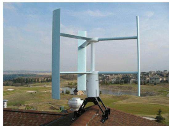
Figure 1: Vertical axis wind turbine (VAWT).
